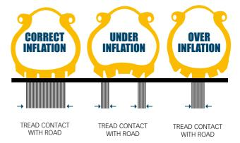
Over-inflation may result in an uncomfortable ride, a reduced area of contact with the road, accelerated wear on the tread centre and makes the tyre more susceptible to impact damage.
