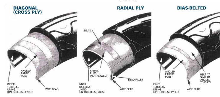
Depending on the wheel type, these may be tubeless (no tube required); or tube type (requiring an inner tube).
